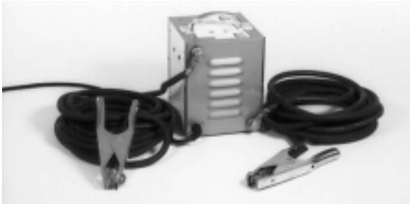
Figure 3 – Thawing Tool with Cables Installed
